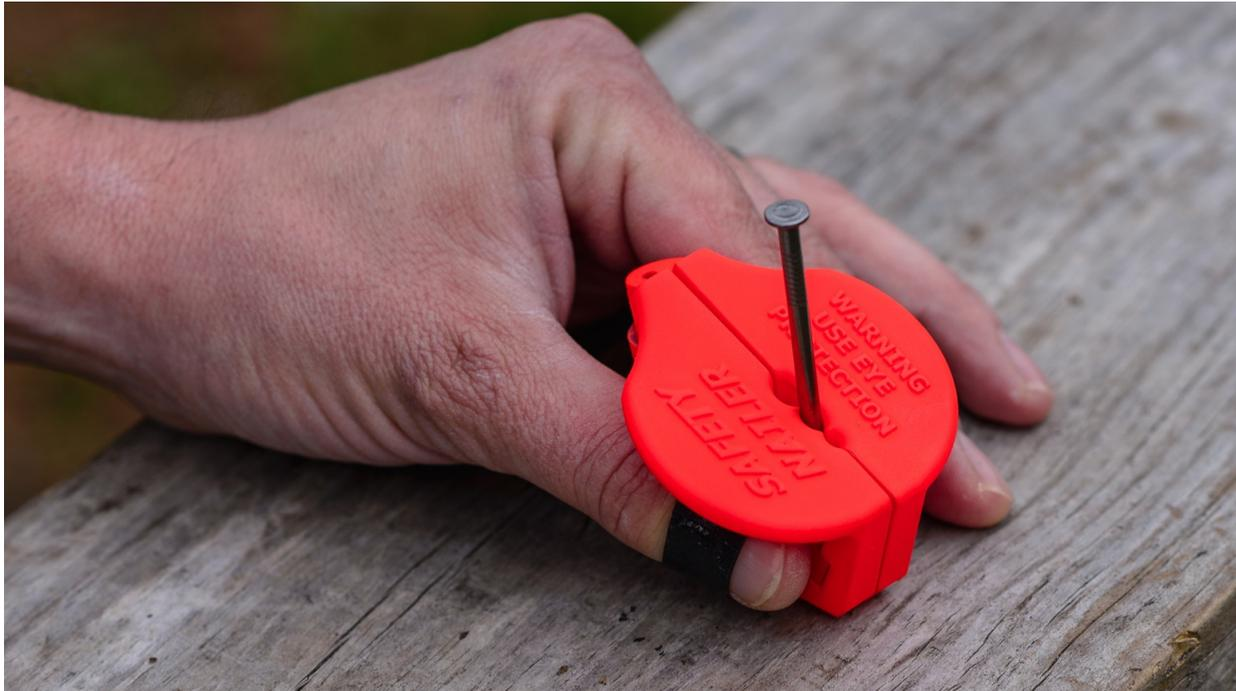
Safety Nailer enables users to hold a nail in place with a smaller risk of striking a finger. (WYDaily/ Courtesy Safety Nailer)
